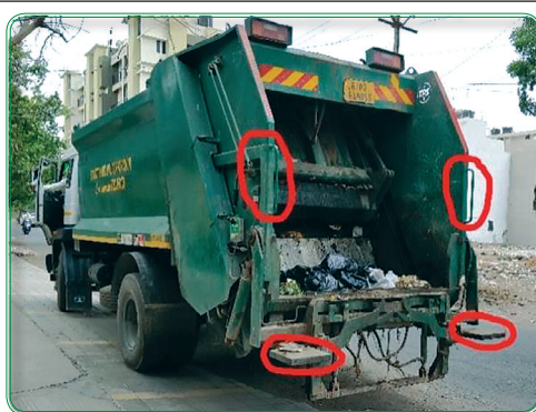
Picture 3: RCV in Rajkot Municipal Corporation with footsteps and hand bars (15.06.2018)
